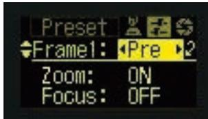
An angle of view can be preset in either of two memories (DD: one memory) and the lens will zoom to that position by pushing a simple button. During a performance, framing preset will reproduce the zoom position decided upon at the rehearsal. It’s easy to repeat the same zoom as often as you like at the highest speed or in a preset zoom speed.
