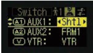
By memorizing any two focal lengths, the Digital Drive can automatically “shuttle” between the two points, moving in either direction.
