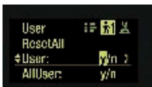
The drive unit can memorize 9 patterns of user-customized settings and also transmit the data between different drive units.
