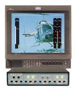
Designed for the non-technical, the PLM1 displays NTSC or PAL Composite video and analog audio levels as coloured bar graphs, which are displayed on screen, mixed or left in the gamut mode. In the gamut mode they are off screen until levels are exceeded, when the appropriate bar graph flashes. Includes also signal loss, non sync., visual, audible alarms and safe area generator. Powered by a PP3 battery or via its 12Vdc adapter (included).
