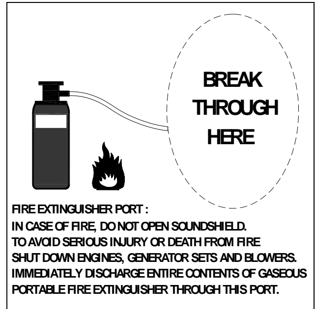
Fig. 2: Fire extinguisher port.
