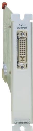
This unit is a DVI-I OUTPUT unit that outputs the contents displayed on the front LCD panel from the DVI-I connector to an external monitor. The unit is installed in a LV 5800 output slot.
